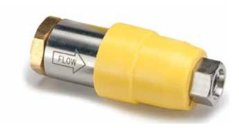
Parker's NGVBCN2-P50 fill line breakaway provides an important safety feature for CNG dispensing systems. It is certified to ANSI/NGV4.4/CSA12.54 standards for breakaway devices used on natural gas dispensing hoses and systems. It allows the hose to safely disconnect, preventing damage to the dispenser in the event of a "drive off" and sealing the CNG in the fill line to effectively prevent leakage or hose whip.
