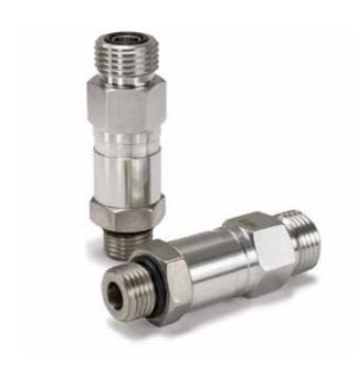
CVS Series check valves provide an important feature for CNG powered vehicles. When installed immediately after the fueling receptacle it functions as a redundant sealing device in the fill line, only allowing flow in one direction, from the dispenser to the vehicle.
